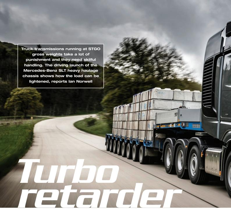
any heavy haulage (HH) operators still rely on manual gearboxes. The fuel penalty of a torque converter fluid coupling is just too much to bear. But now they have a new device to consider: the turbo retarder clutch, or TRC, an early version of which made a stealthy debut as an option on the predecessor to Mercedes-Benz's new SLT range, the Titan.
